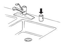
The drain air gap is usually located on top of the sink or countertop near the dishwasher. To order a drain air gap, please call **1-800-4-MY-HOME**<sup>®</sup>. Ask for Part Number 300096.
